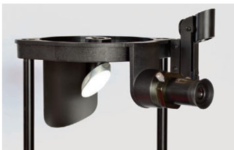
A key element in the telescope's baffling is a plastic shield located opposite the focuser. This worked reasonably well, but the shield was a bit too small to be completely effective in bright environments.
