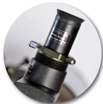
Unlike similar tabletop reflectors, OneSky has a nifty helical focuser rather than a rack-and-pinion model. It is excellent for fine-tuning the focus, especially at high magnifications, but there was enough play in the helical threads to let the eyepiece go out of focus when the scope was moved through a large sweep in elevation.
