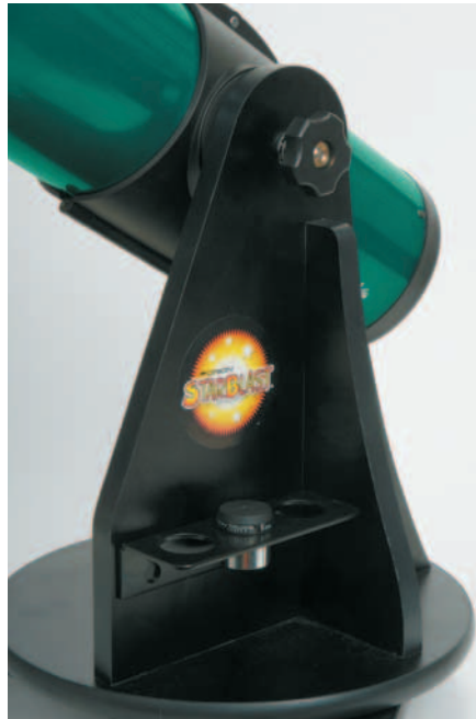
Above, left: The StarBlast's optical tube is cradled in a hinged, felt-lined metal clamp that can be readily adjusted with a single easily gripped thumbscrew. Not only can the tube be removed from the mount for cleaning or storage; it can be rotated to optimize the eyepiece angle. What's more, it can be balanced even if an unusually heavy eyepiece is placed in the focuser. Above, right: Among the many conveniences of the StarBlast's stable, sturdy altazimuth mount are an eyepiece rack and a knob for adjusting the friction in the altitude (up-and-down) axis.
