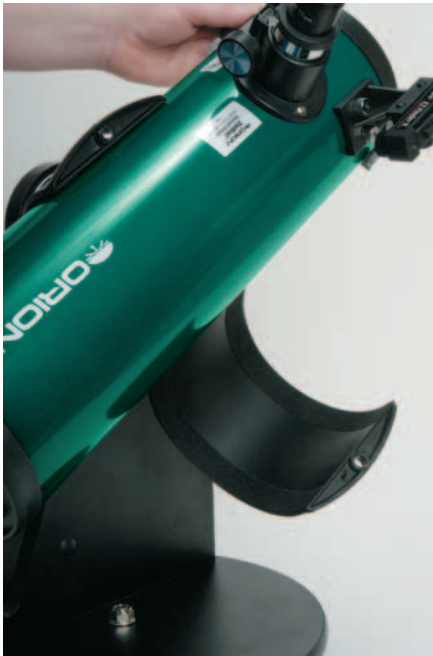
Above, left: The StarBlast's optical tube is cradled in a hinged, felt-lined metal clamp that can be readily adjusted with a single easily gripped thumbscrew. Not only can the tube be removed from the mount for cleaning or storage; it can be rotated to optimize the eyepiece angle. What's more, it can be balanced even if an unusually heavy eyepiece is placed in the focuser. Above, right: Among the many conveniences of the StarBlast's stable, sturdy altazimuth mount are an eyepiece rack and a knob for adjusting the friction in the altitude (up-and-down) axis.
