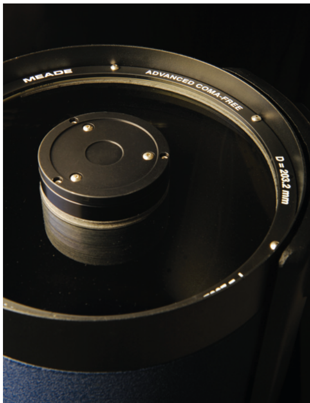
LightSwitch telescopes are available with either Meade's traditional Schmidt-Cassegrain optics or the newer and somewhat more costly advanced coma-free design, which offers improved image quality at the edge of the field of view.
