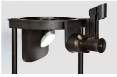
A key element in the telescope's baffling is a plastic shield located opposite the focuser. This worked reasonably well, but the shield was a bit too small to be completely effective in bright environments.
