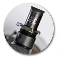
Unlike similar tabletop reflectors, OneSky has a nifty helical focuser rather than a rack-and-pinion model. It is excellent for fine-tuning the focus, especially at high magnifications, but there was enough play in the helical threads to let the eyepiece go out of focus when the scope was moved through a large sweep in elevation.
