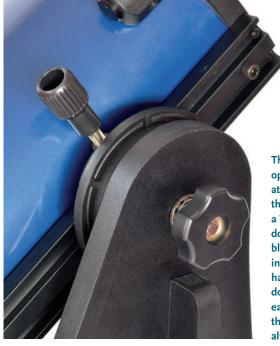
The scope's optical tube attaches to the mount via a Vixen-style dovetail assembly, which locks in place with a hand knob. The dovetail lets you easily balance the scope on its altitude axis.
