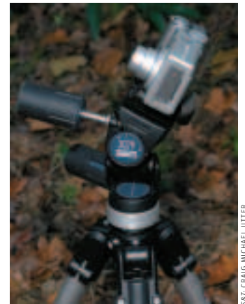
Any digital camera that can take multisecond exposures under full manual control can measure suburban skyglow. The angle scales on this pan/tilt head make it easy to take the sequence of shots needed for full-sky coverage, but the author frequently meters the zenith just by setting the camera on the ground with its lens pointing up.
