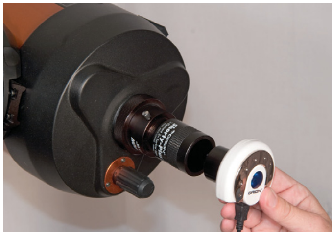
Planetary webcams available today come equipped with a 1¼-inch nosepiece and fit directly into your telescope's focuser. To increase the magnification, Barlow lenses, tele-extendors, or eyepieces are placed between the telescope and camera. Photo: Alan Dyer
