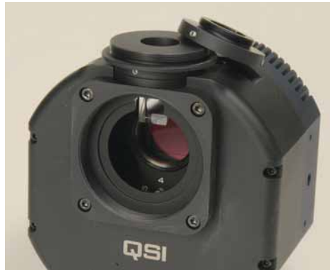
The off-axis guider port uses a generous ½-inch-square prism and an adjustable focusing mechanism for autoguiders. Adapters are available for autoguiders with standard T mounts (shown attached) as well as CS/C mounts.
