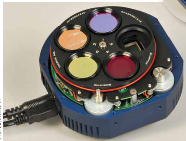
Despite its compact body dimensions, the QSI 540wsg includes a mechanical shutter and five-position filter wheel.
