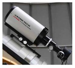
The author tested the QSI 540wsg CCD camera with an Astro-Tech AT6RC Ritchey-Chrétien telescope piggybacked on Phillips Academy Observatory's 16-inch DFM Engineering classical Cassegrain telescope.
