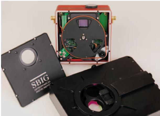
**The filter wheel** attaches to the STT-8300 after removing the camera's front cover. A new design ensures that filters precisely return to the same position each time they are moved, which is critical for flat-fielding images when dust is on the filters. The self-guiding mechanism visible at lower right is described in the text.
