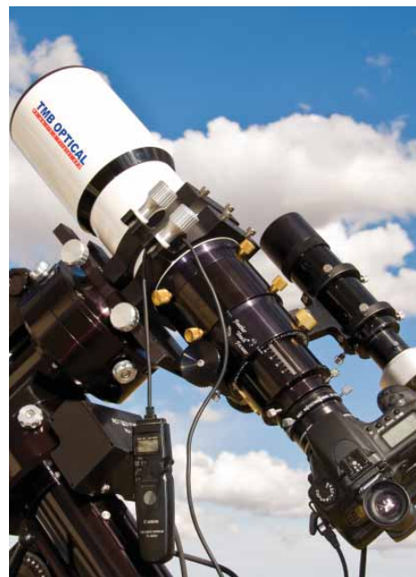
The TMB-92 fitted with a Borg 0.85× field flattener and camera adapter, an Orion Autoguider on a 50-mm finder/guidescope, and an Astro-Physics Mach 1 mount served as the astrophotography platform that the author used for his Canon 20Da DSLR camera.
