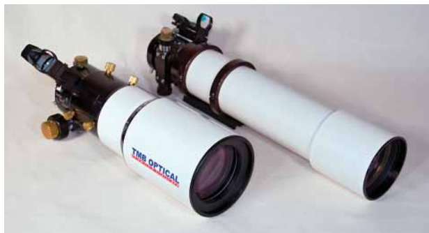
The author star-tested the TMB-92 (left) against his limited-edition Astro-Physics 92-mm f/7 Stowaway (right), an instrument that has become the gold standard for small apo refractors.
