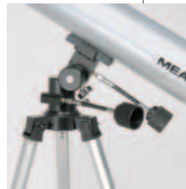
The Meade 3-inch reflector came with the nicest altazimuth mount — one that features heavy-duty construction and slow-motion controls for both axes. Unfortunately, this fine system was hobbled by an inadequate tripod that quivered at the slightest touch.
