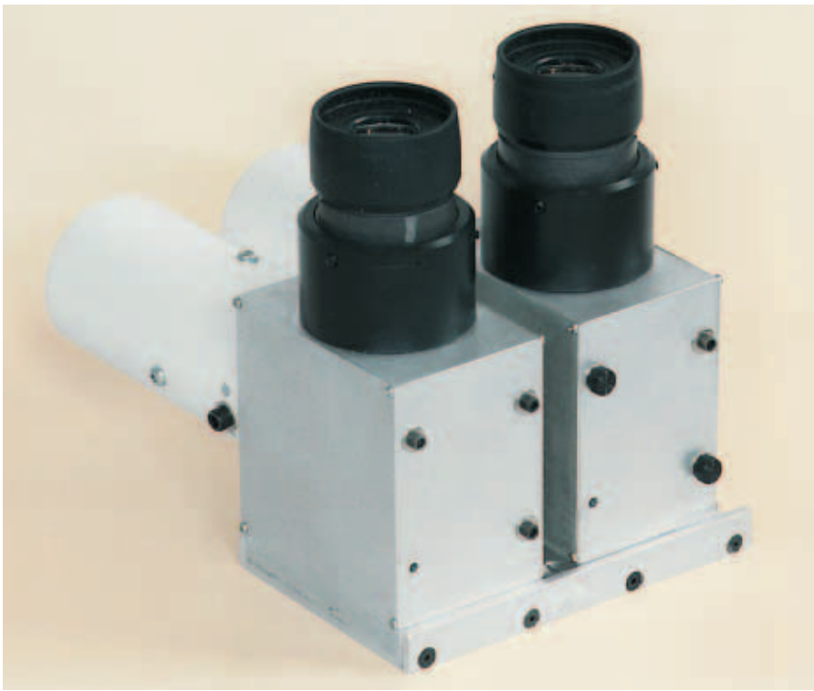
LeDrew's binoculars consist of a pair of carefully aligned optical trains, each having an eyepiece, Amici prism, and objective lens.
