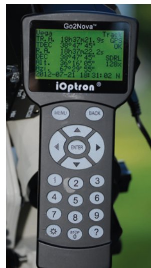
A robust screw ( left ) provides precise adjustment of the polar-axis altitude. The hand control's 8-line display ( right ) also shows the location of Polaris on the polar-alignment reticle when the mount is properly aligned ( below ).
