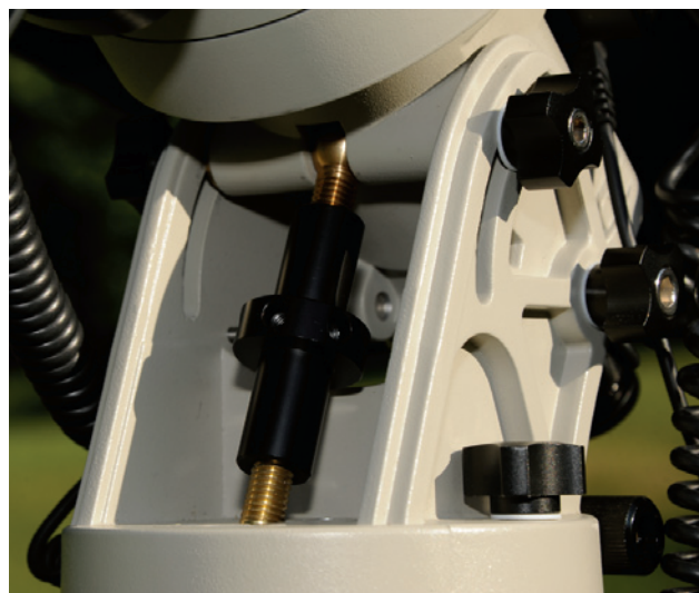
A robust screw ( left ) provides precise adjustment of the polar-axis altitude. The hand control's 8-line display ( right ) also shows the location of Polaris on the polar-alignment reticle when the mount is properly aligned ( below ).
