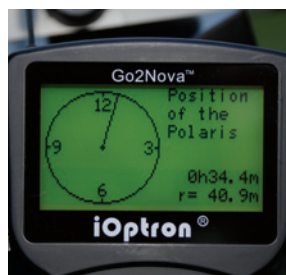
A robust screw ( left ) provides precise adjustment of the polar-axis altitude. The hand control's 8-line display ( right ) also shows the location of Polaris on the polar-alignment reticle when the mount is properly aligned ( below ).
